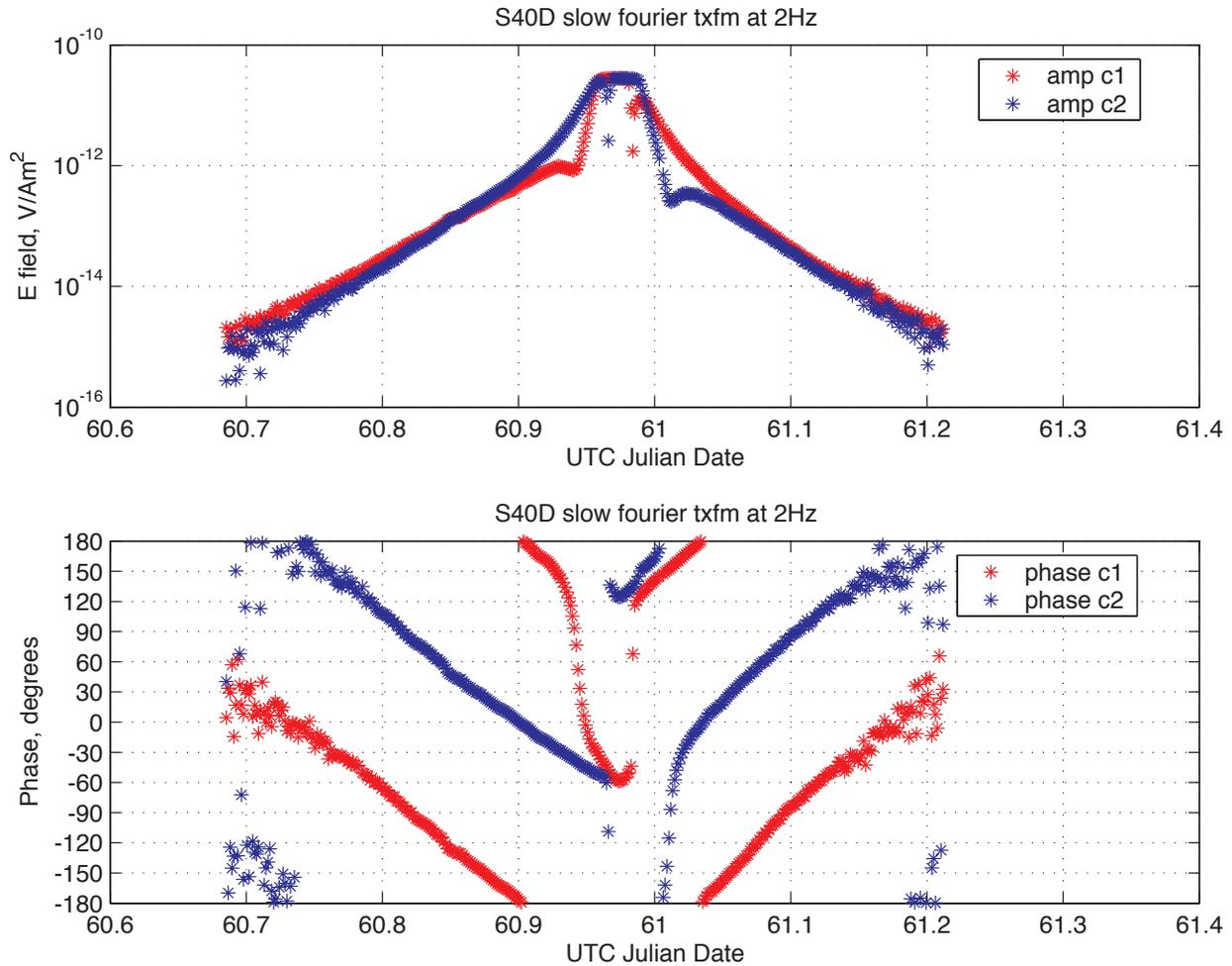
Figure 6. Controlled source transmission from the entire tow 4 into Bandicoot, site S40. Note the excellent stability in amplitude and phase, and noise floor of  $10^{-15}$  V/m/Am. The time axis of 0.5 days corresponds to about 30 km.
