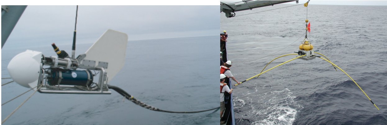
Figure 4: Left: SUESI-200, the second-generation EM transmitter being deployed. This unit has a 200 A output (a 500 A version is now available). Right: A receiver instrument being deployed. A total of 45 such receivers are currently available.
