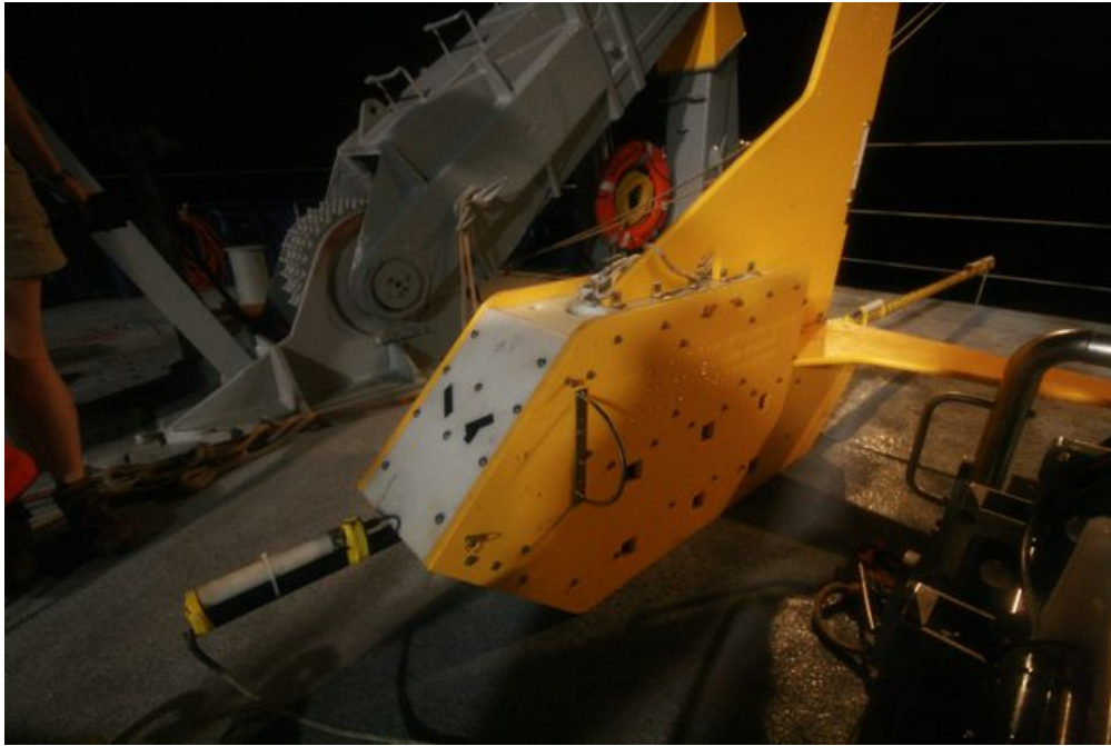
Figure 8: Vulcan, the towed 3-axis electric field receiver, on deck during the SERPENT cruise.
