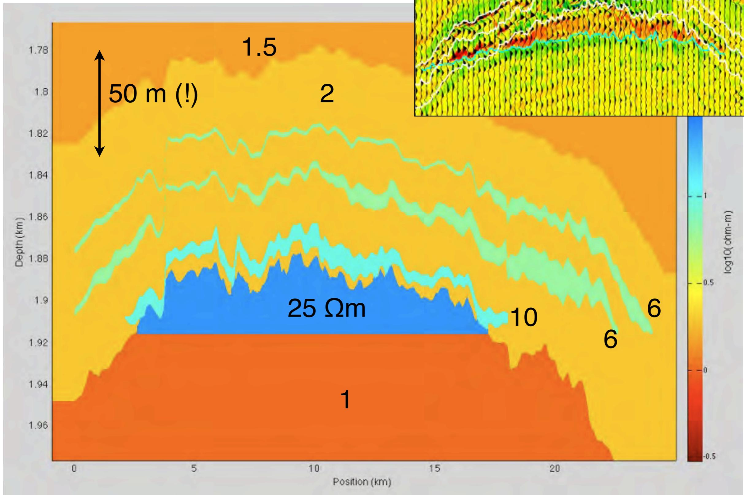
Ey, Ez and Bx at 0.1 and 1 Hz inverted with OCCAM1D after adding 1% random noise and omitting data below noise floor:
