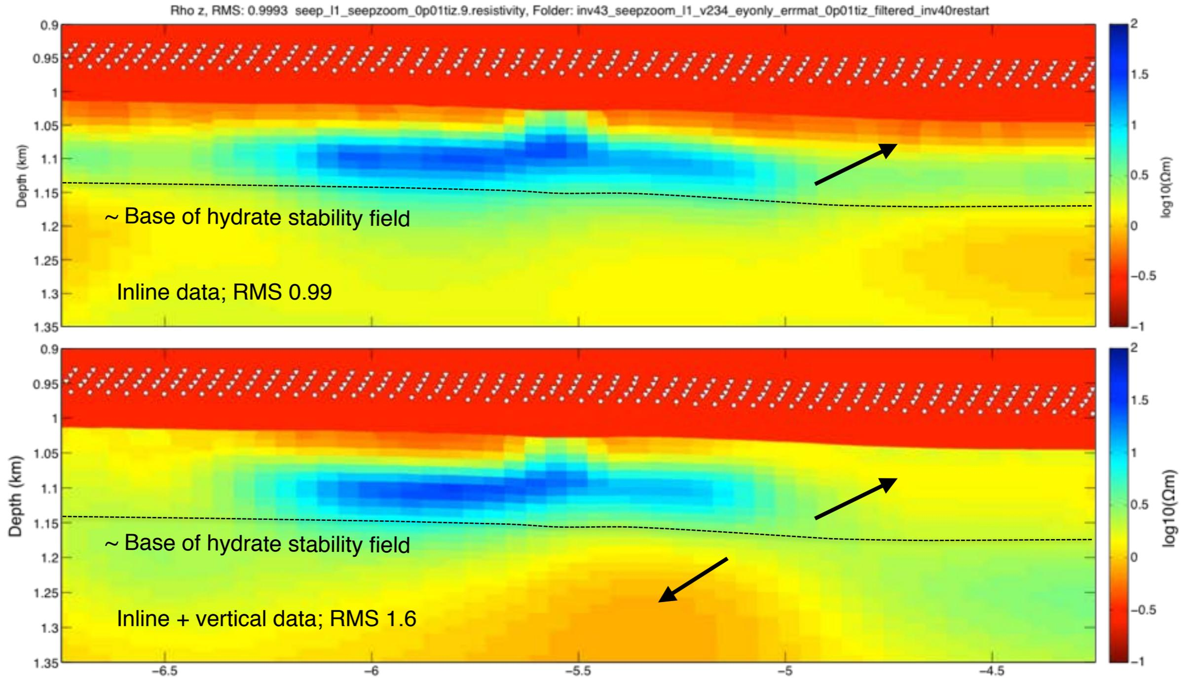
Anisotropy (ratio of vertical to horizontal resistivities) is very high in the northern part of the region inferred to be gas hydrate.
