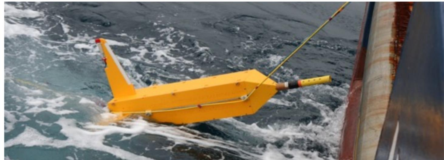
Voltage noise is comparable to our seafloor instrument. (But, dipoles are 5-10 times shorter.)
