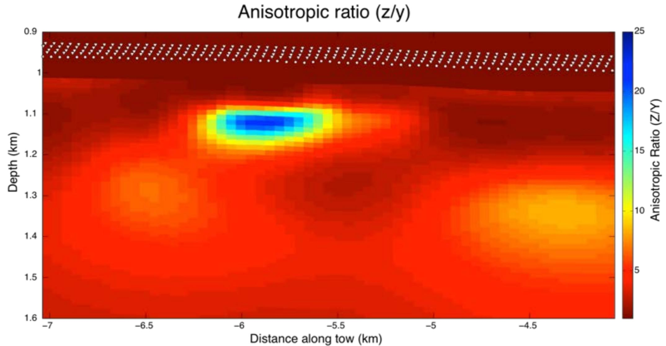
Using Archie's Law, resistivity can be converted to hydrate saturation. Integrating saturation provides an estimate of 2 billion cubic meters of methane, or 0.07 tcf.
