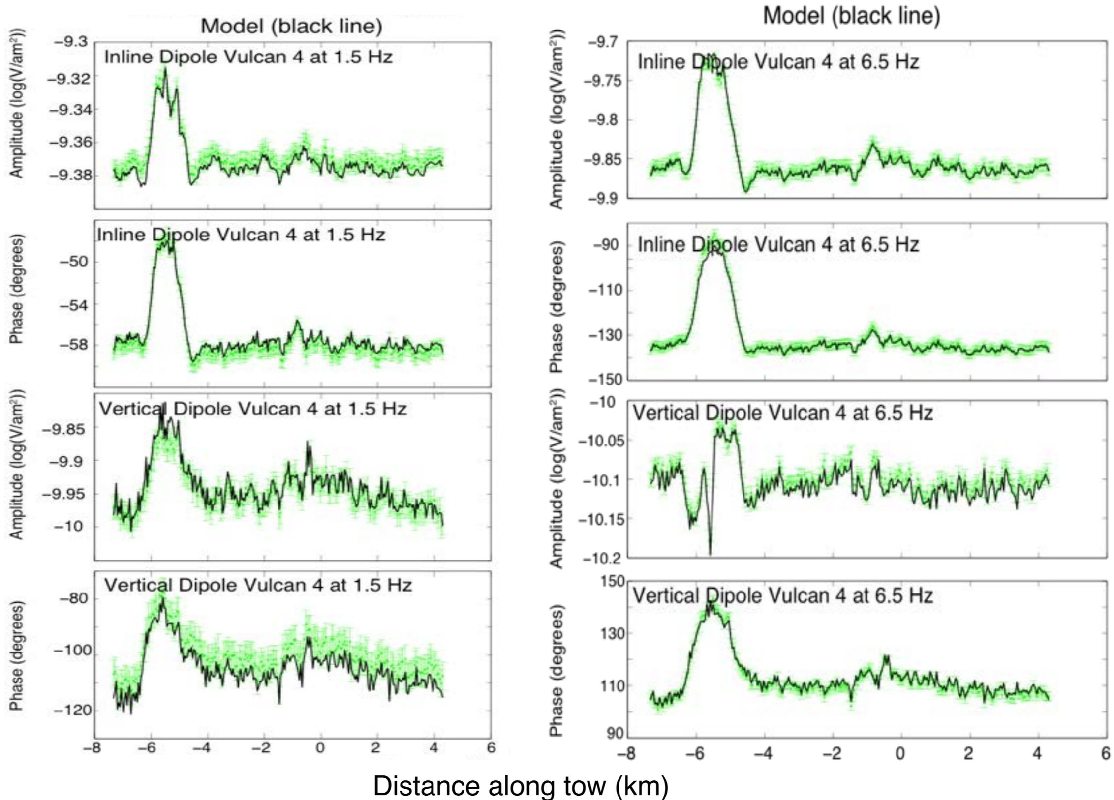
Addition of the vertical electric field data removes what appears to be a layering artifact and brings out a conductor that may be fluids feeding the vent.
