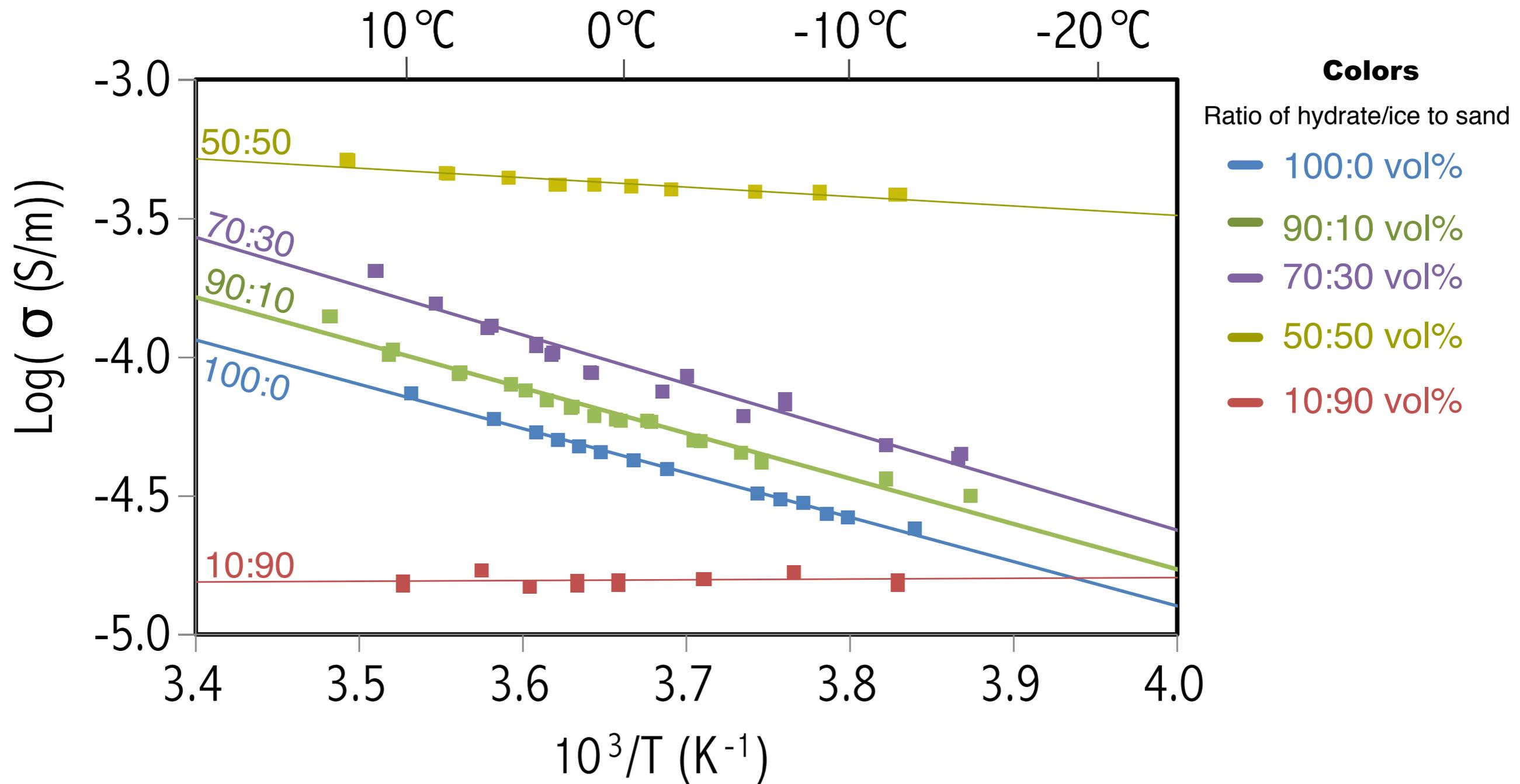
Mixed with silica sand, hydrate conductivity goes up until a percolation threshold is reached. We think that impurities from the sand, probably  $K^+$  and  $Cl^-$ , increase the charge carriers available in the hydrate.
