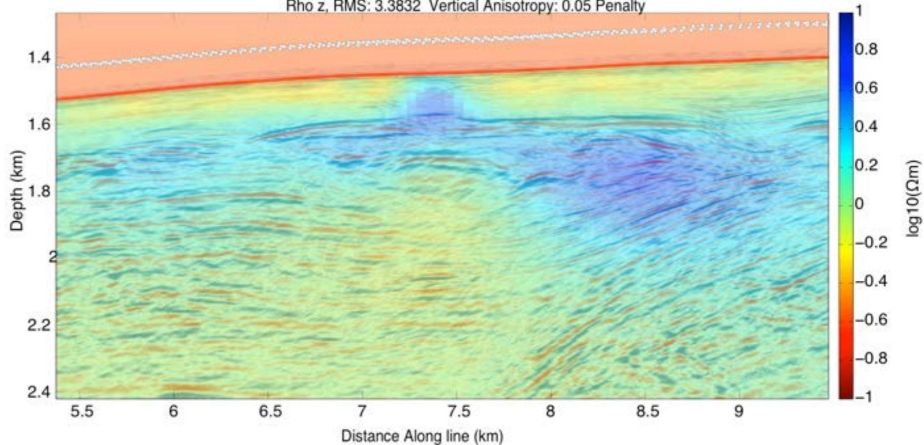
~8  $\Omega\text{m}$  resistor lies entirely above the BSR, while a resistor to the east lies under (gas?)
