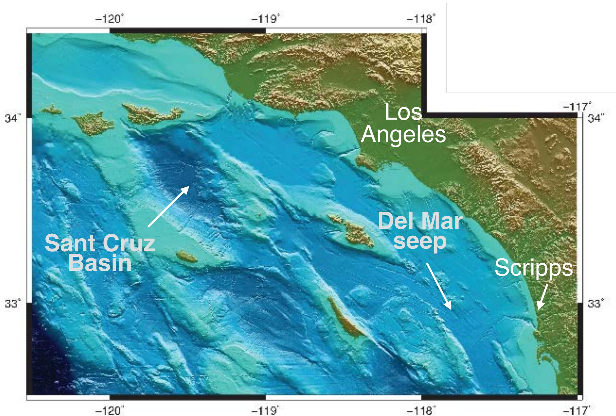
The Del Mar seep is a methane vent in the San Diego Trough, studied by Scripps students. It is in a pop-up structure bounded by two strands of the San Diego Trough Fault.
