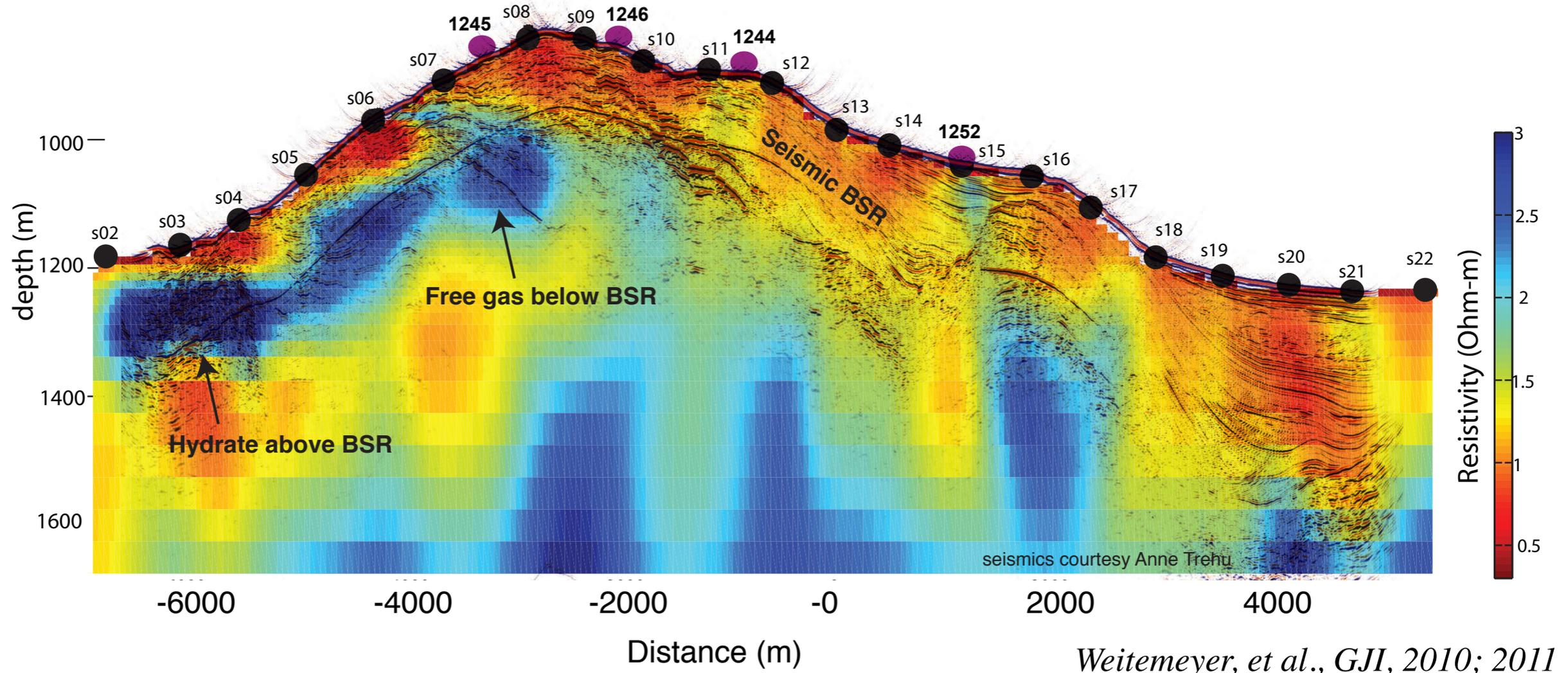
High resistivity below the BSR corresponds to low seismic velocities  $\rightarrow$  free gas, while high resistivity above the BSR suggests hydrate.
