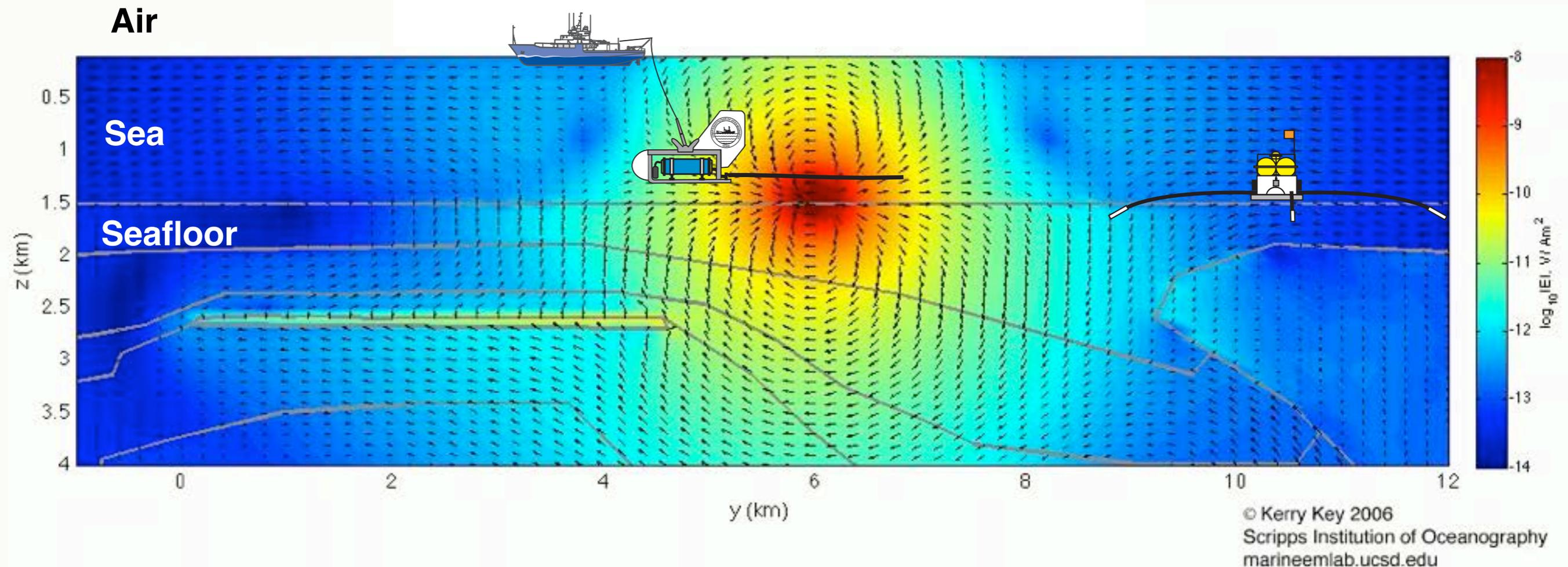
Amplitude and phase of the magnetic/electric fields on the seafloor can be used to infer geological structure to depths of several km.
