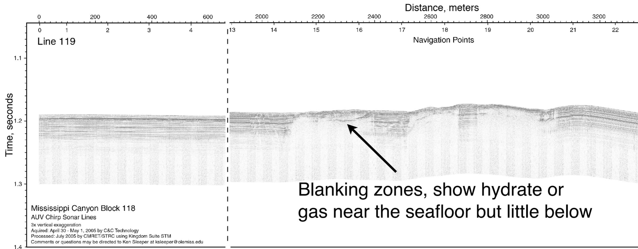
The BSR reflection is associated with small amounts of free gas - similar to the “fizz-gas” problem in hydrocarbon exploration.
