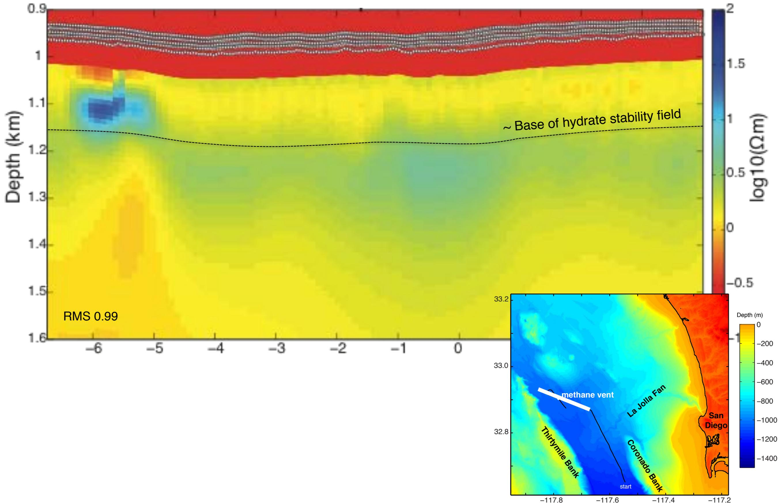
Frequencies of 1.5, 3.5, 6.5 Hz were fit for 3 Vulcans. Ey fits to 1% amplitude and  $0.6^\circ$  phase. As predicted, there is a strong low-frequency signal in Ez.
