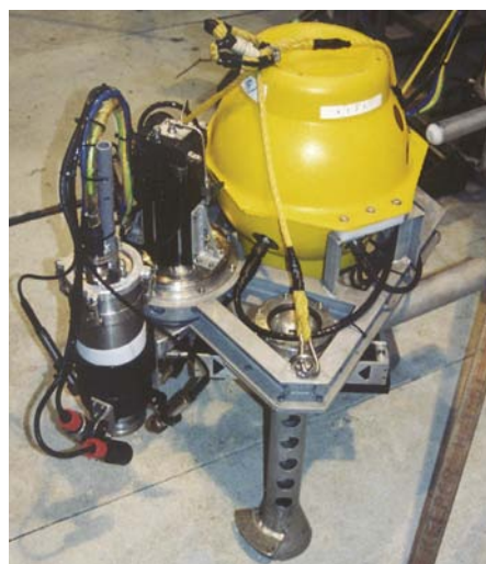
Fig. 1. (left) The DORISS instrument is a Kaiser Optical Systems laser Raman spectrometer modified for deep-ocean use and divided into three 4000 m-rated pressure housings (modified from Brewer et al. , 2004). (right) The Precision Underwater Positioner (PUP) is used to position the DORISS probe head (mounted at left) with a precision of ~0.1 mm.
