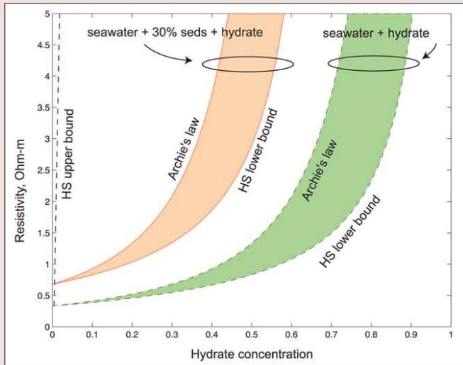
**Figure 6.** Archie's law, and Hashin-Shtrikman (HS) upper and lower bounds for a hydrate and seawater mix, and for a hydrate, seawater, and sediment mix. It is likely that the hydrate resistivity falls between Archie's law and the HS lower bound. The HS upper bound is unlikely to be a useful model but is included for completeness.
