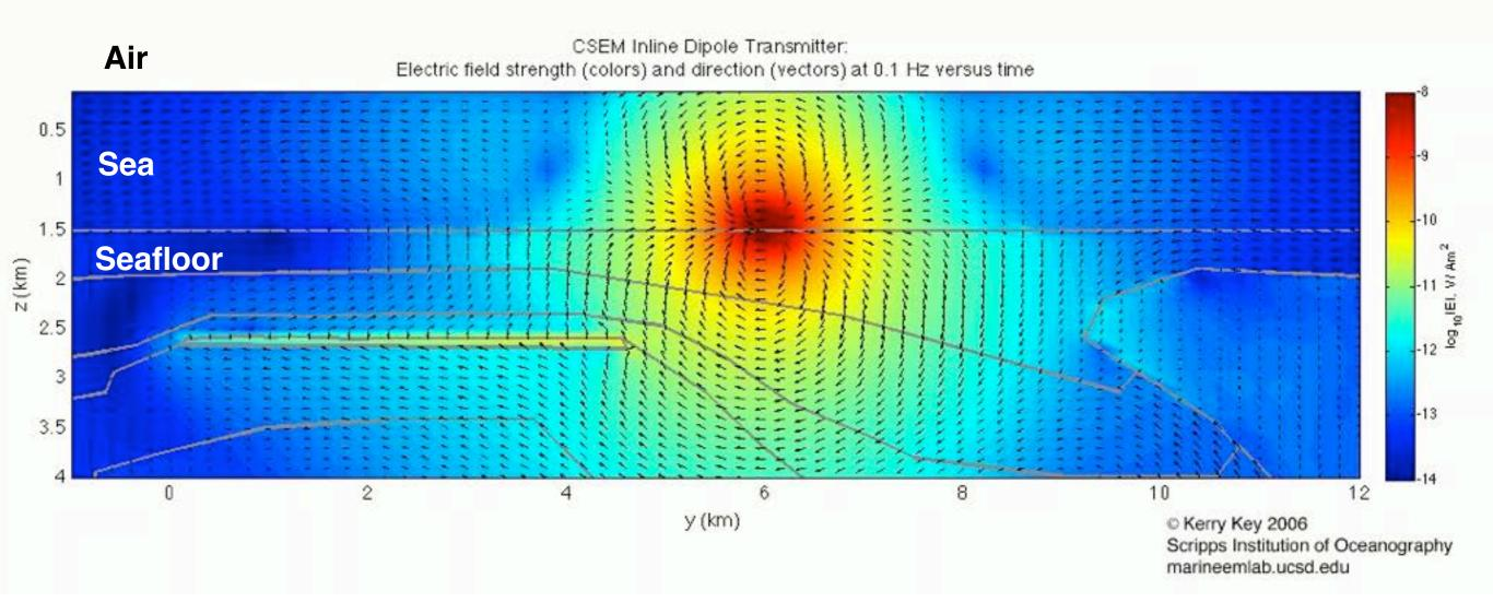
With frequency domain CSEM, the entire air-sea-seafloor system is illuminated continuously. Energy propagates preferentially in resistive rocks.
