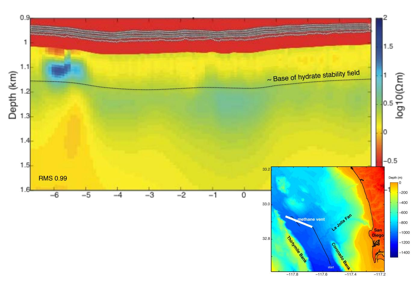
Frequencies of 1.5, 3.5, 6.5 Hz were fit for 3 Vulcans. Ey fits to 1% amplitude and 0.6° phase. As predicted, there is a strong low-frequency signal in Ez.
