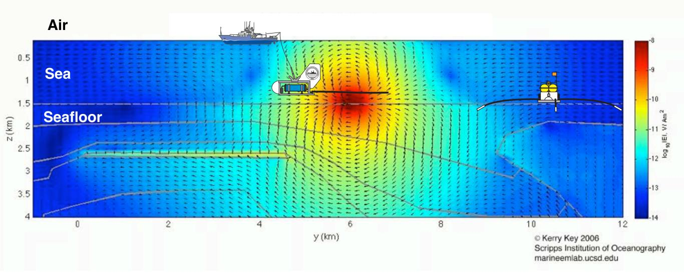
Amplitude and phase of the magnetic/electric fields on the seafloor can be used to infer geological structure to depths of several km.
