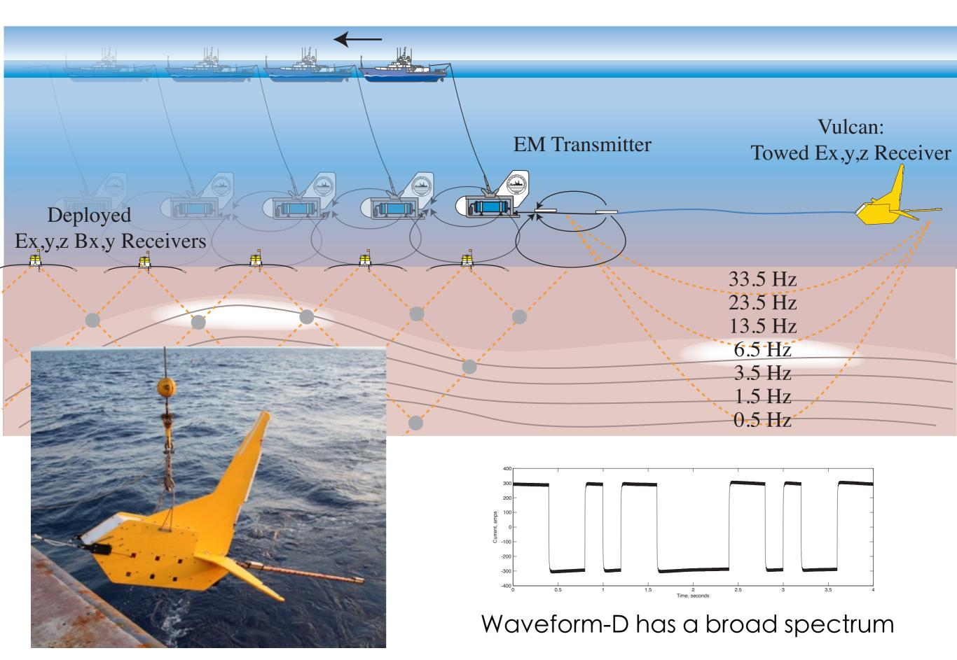
MC 118, Gulf of Mexico using seafloor instruments and towed receiver:
