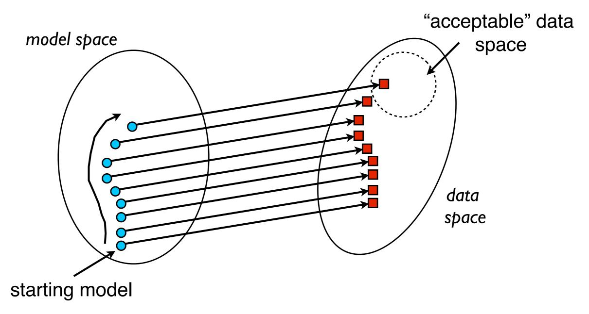
The direction of the search is determined by how changing parts of the model affects the fit to the data.
