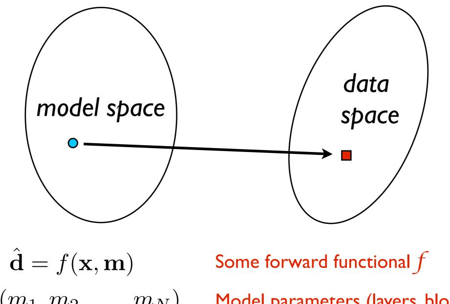
$\mathbf{m} = (m_1, m_2, \dots, m_N) \qquad \text{Model parameters (layers, blocks, ...)}$  $\mathbf{x} = (x_1, x_2, x_3, \dots, x_{kM}) \quad \text{Independent variables (freqs., locations, ...)}$  $\hat{\mathbf{d}} = (\hat{d}_1, \hat{d}_2, \hat{d}_3, \dots, \hat{d}_M) \quad \text{Predicted data (gravity, magnetic, electric, ...)}$
