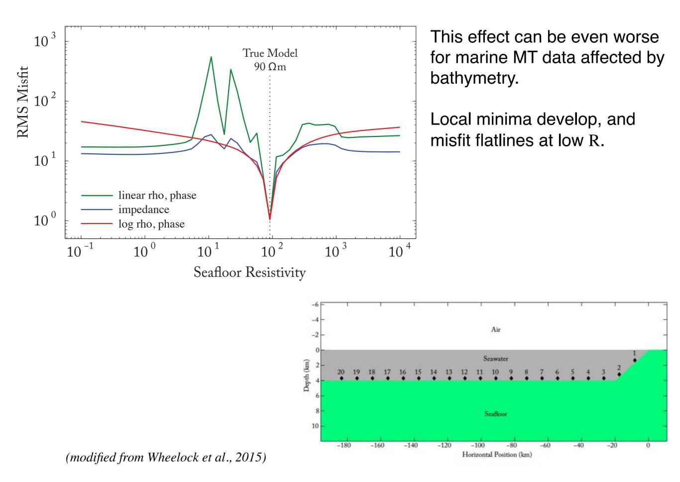
Here is a 2D example. Linear apparent resistivity and phase converged, but log(resistivity) converges to the same model in half the iterations. MT impedance, Z, did not converge (d.n.c) at all.
