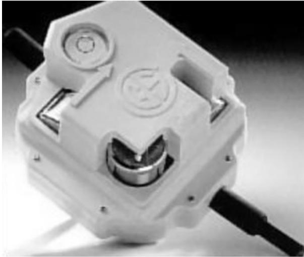
Fig. 4.40 A three-component geophone.
