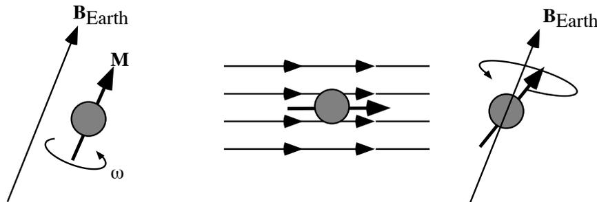
Fig.M.17: The operation of a proton precession magnetometer.
