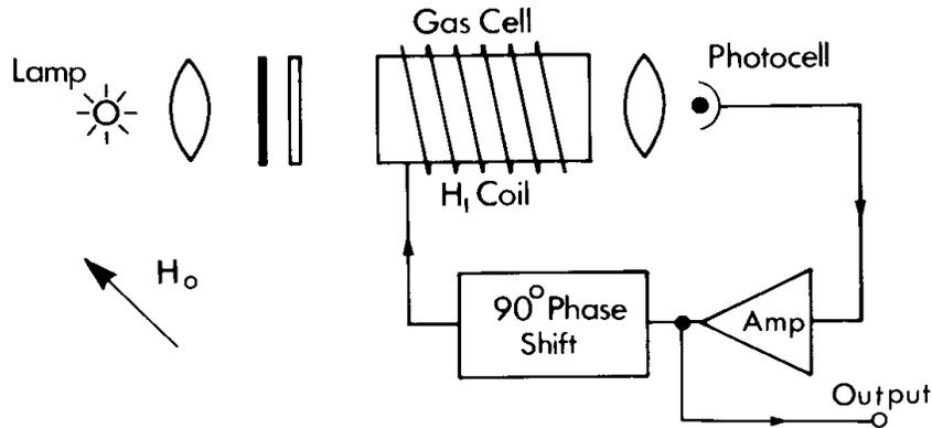
Fig.M.19: Schematic of a self-oscillating alkali vapour magnetometer (from Forbes, 1987).
