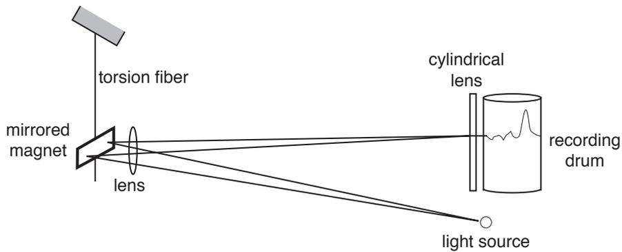
Fig.M.16: Schematic of a torsion fiber magnetometer.
