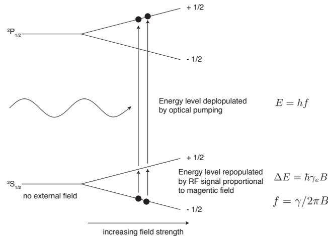
Fig.M.18: Zeeman splitting of the energy level of the valence electron & optical pumping.
