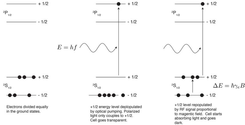
Fig.M.18: Zeeman splitting of the energy level of the valence electron & optical pumping.
