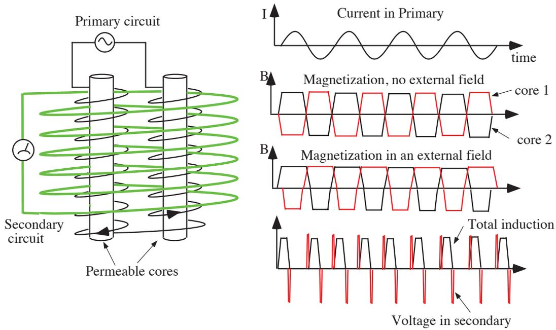
Fig.M.21: Fluxgate magnetometer.
