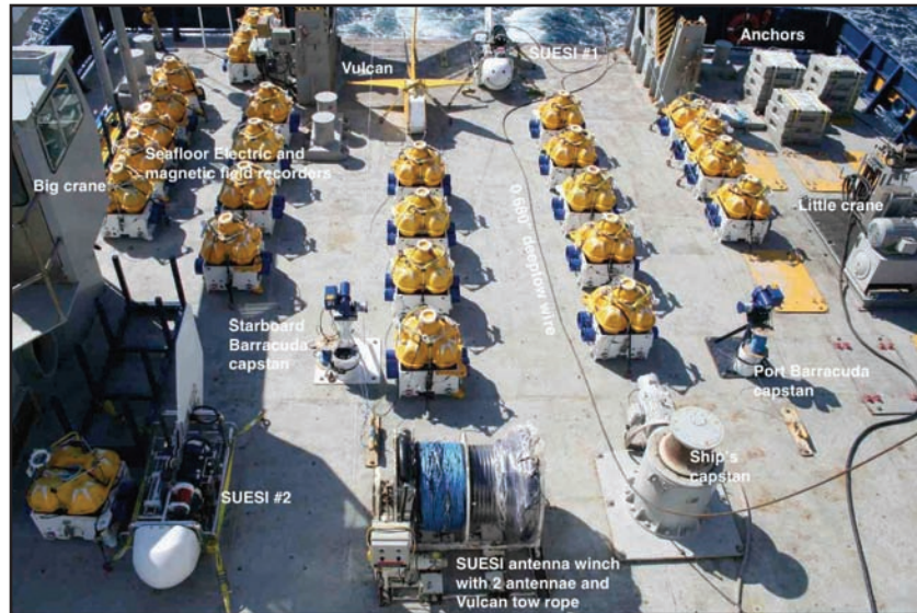
Figure 3: Deck of R.V. Roger Revelle showing instruments used for this survey.
